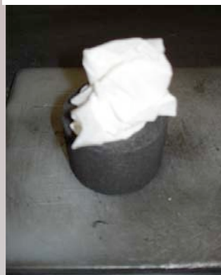
Kimwipe + compressed air cleaning
